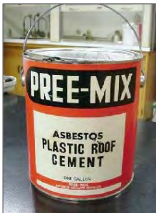
Asbestos Roof Cement
